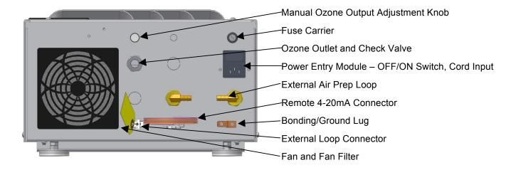
Shown: ClearWater Tech CD12/AD Ozone Generator (Wire harness omitted for clarity)
